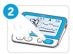
While the device is off, press the "Start/Stop" button. The cuff around your arm will automatically inflate and stop once the measurement is complete.
